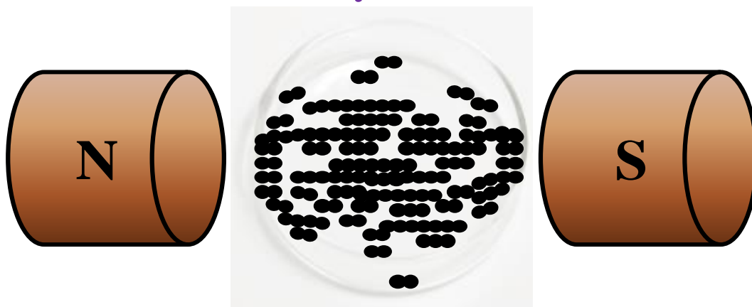
Fig. 4.3: Schematic of magnetic alignment of nickel nanostructures
